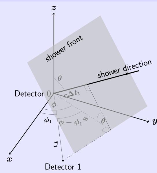
When an inclined shower front passes over the station, it will hit detectors at different times. The shower direction can be calculated using
