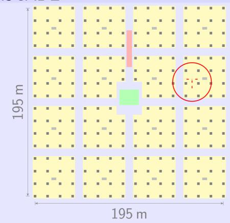
The KASCADE array contains 252 detector huts placed 13 m apart. The HiSPARC station is drawn in red. The KASCADE array is able to pinpoint the direction of the shower to within  $0.1^{\circ}$ .
