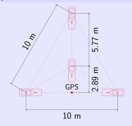
A HiSPARC station consisting of four detectors is placed in an equilateral triangle. The electronics must be able to pick up time differences which are only a few nanoseconds. The GPS unit provides an accurate timestamp to individual events.
