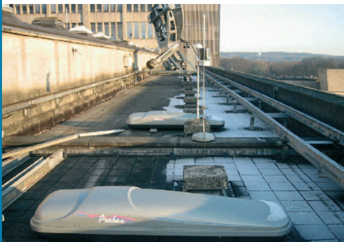
▲ Fig. 3: Twin particle detector station on top of the building of the Radboud University Nijmegen. The ski boxes accommodate scintillator plates connected to a photo multiplier tube (PMT). The two poles between the ski boxes carry a weather station and the GPS for timing information. An analog signal cable runs from each box to the coincidence electronics.
