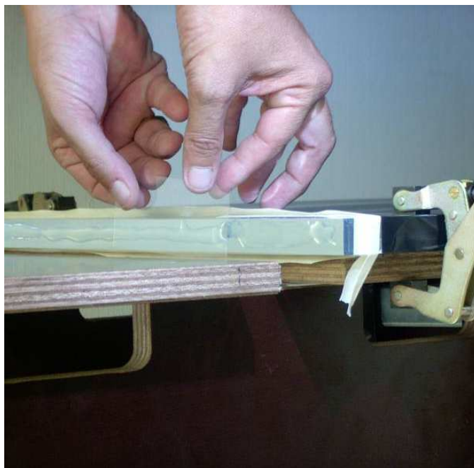
Figure 20: Spread the glue with a plastic card
