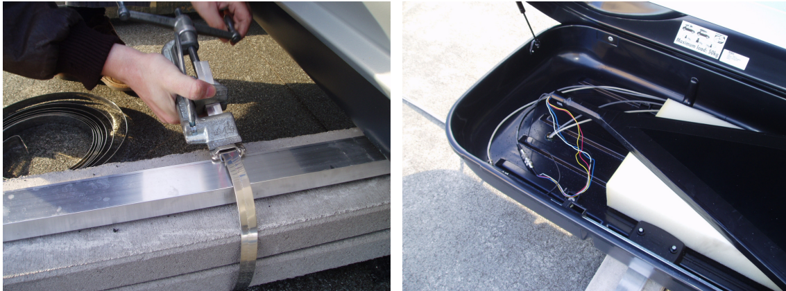
Figure 4.5: Another detail of the attachment link and attachment grip (left). The detector is put back into the box and is supported by plastic foam (right).
