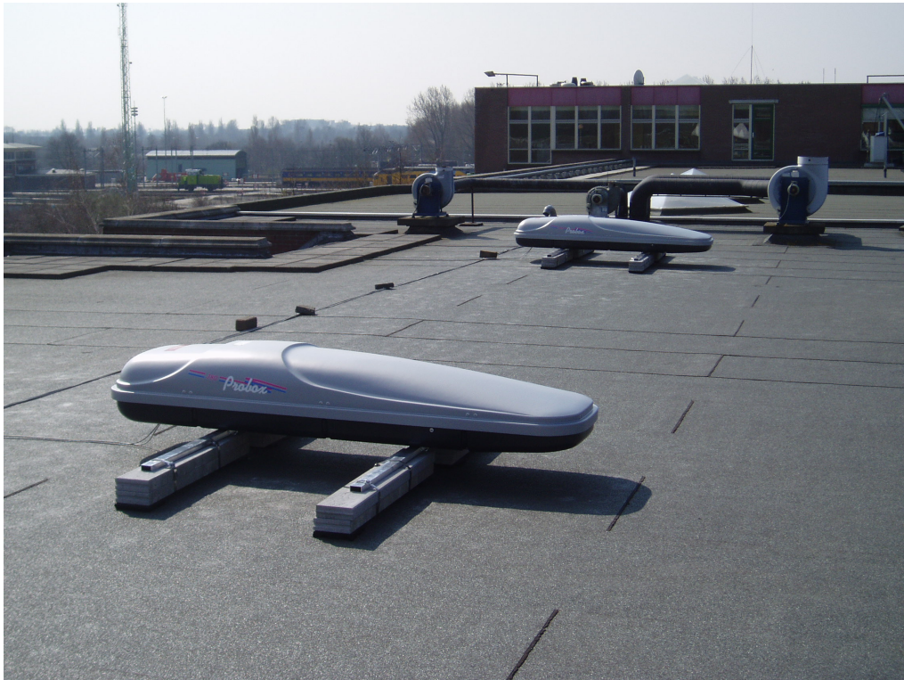
Figure 1.1: HiSPARC detector with two ski boxes.
