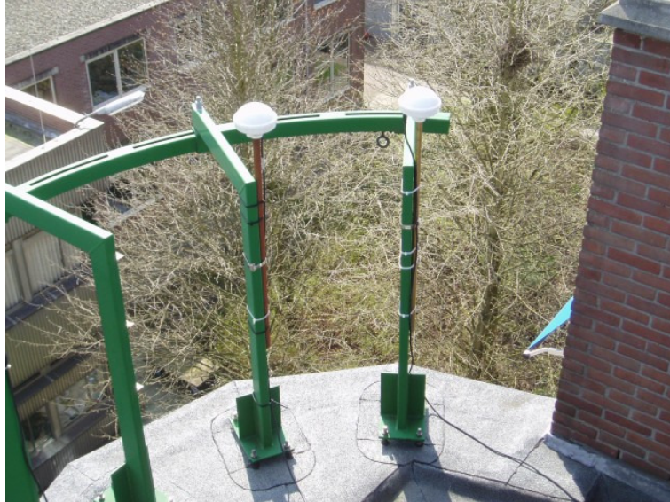
Figure 3.1: Please pay attention! Working on a roof requires keeping a distance of 2 meters to the edges! Optionally place the GPS on a stable tube or use the plastic antenna anchor. Do not leave the cable hanging freely off the antenna.
