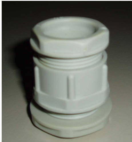
Figure 3.2: The cable transit is plugged into the hole in the bottom of the ski box in the vicinity of the PMT. The bulk of the transit sits inside the ski box; only the nut at the bottom of the image above will sit outside the ski box..
