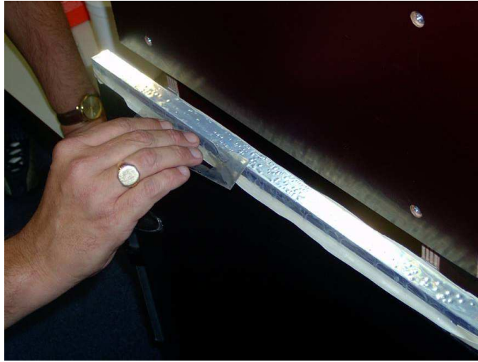
Figure 21: Bubbles during gluing
